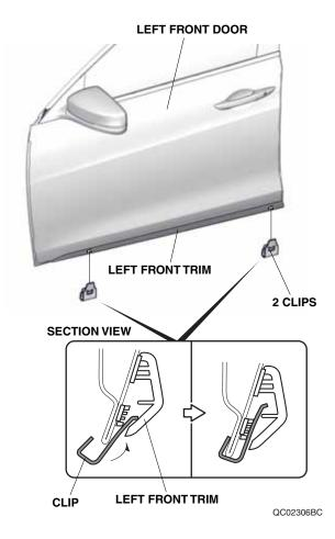
6. Using a rubber roller, apply firm pressure against the trim and roll from one end to the other. Apply firm pressure, especially at the ends.
